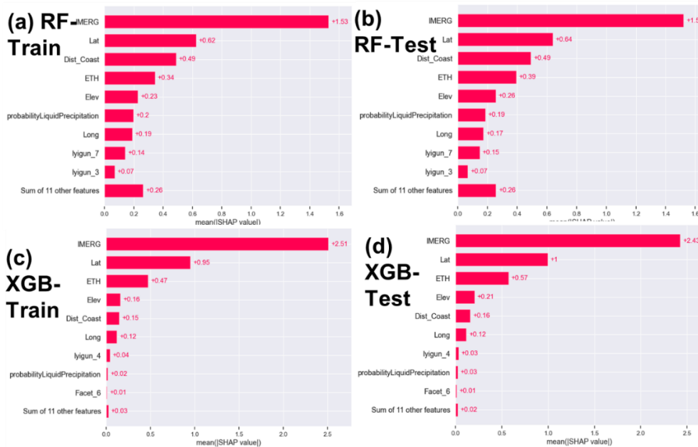
Figure 4.4. SHAP absolute mean plots (Feature Importance) for Random Forest (a) Train dataset, (b) Test dataset and XGBoost (c) Train Dataset (d) Test Dataset (selected day: 16/11/2018)
